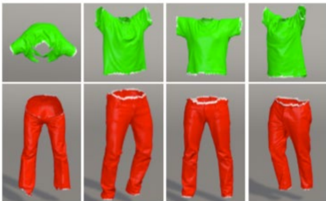
Fig. 7. Segmentation results: rows of scan geometry segmentations, shirt (top row), pants (bottom row). After solving the discrete MRF on the body topology we propagate the obtained labels back to the scan. This results in segmented scans S_k . Boundaries (shown in white) can be easily identified and are propagated to the scans. Such labels provide important information for the multi-cloth alignment step. They allow ClothCap to estimate consistent geometry with smooth boundaries.
